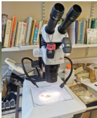
Microscope set up used to identify insects caught in the Rothamsted Insect Survey suction-trap. Each insect is individually and manually identified and counted using taxonomic keys
